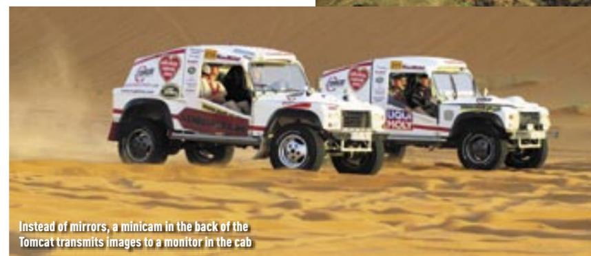
Instead of mirrors, a minicam in the back of the Tomcat transmits images to a monitor in the cab
